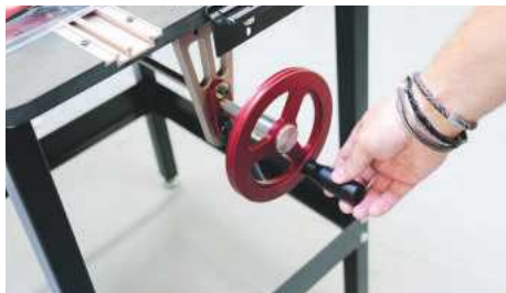
▲ Height adjustments are fluid and free of backlash with the side handle
